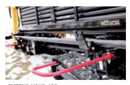
**EXTEND YOUR JOB.** Increase the length of your bore and minimize the loading time with the semiautomated add-a-rod feature. Add more rods [10' (3.1 m) rod] to maximize jobsite productivity.
