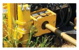
KEEP YOUR TORQUE IN CHECK. The torque limiter provides proper makeup torque to drill rod joints, and prevents operator from over-torquing drill rod, helping to increase life of the drive chuck and drill rod.
