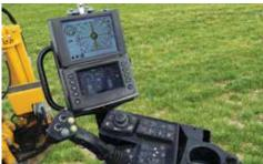
DRILL EFFICIENTLY. The D24x40 Series II features the DigiTrak® Aurora™ full-color touchscreen display, delivering real-time, easy-to-view locate information which can help make a driller's day more productive.
